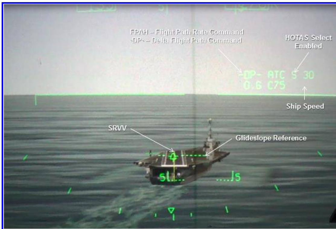
Figure 3. Head-Up Display Symbology for Carrier Landing
